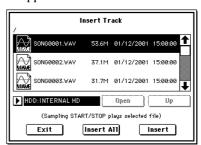
Use "Drive select" to select the drive (internal hard disk, etc.) that contains the file you want to add, use the Open button and Up button to move to the desired directory, and select the WAVE file. (1880-1c, 0-1d)
